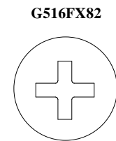
G516FX82 Philips screw head G5-16 with body 82 mm long - front
