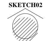
Substaion or distribution center, indoor - in service
