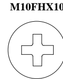
M10FHX10 Philips screw head M10 with body 100 mm long - front
