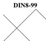
Lighting outlet with circuit breaker
